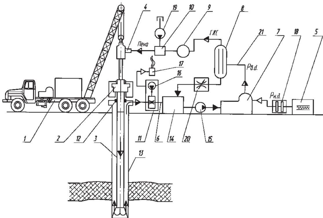
Picture 2 – The layout of location of equipment complement with output washing of productive strings by the foam:
