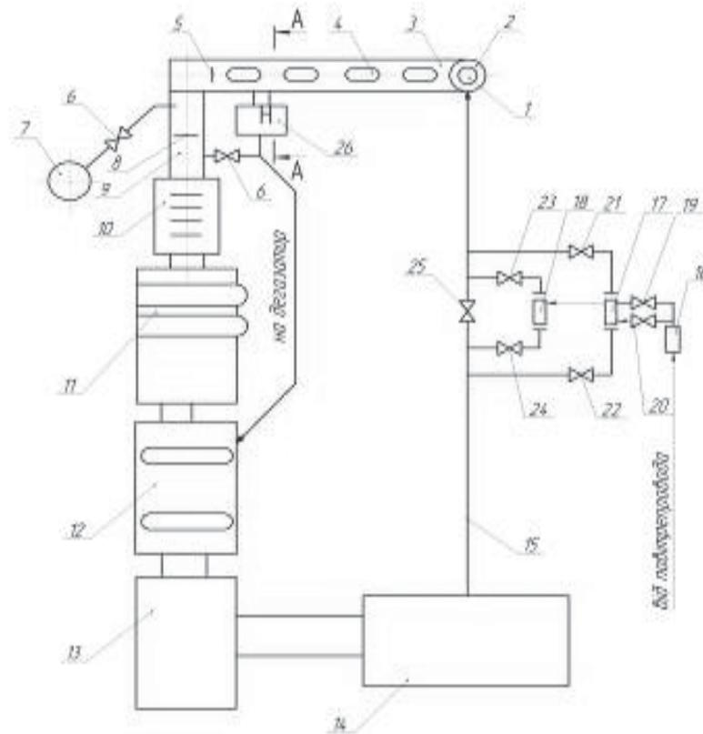
*Picture 3 – The layout of strapping of circulated system during drilling with well washing by the foam:*
