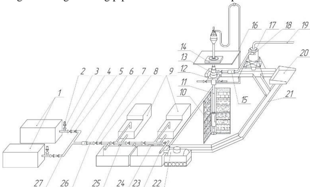
*Picture 1 – The principal scheme of equipment strapping for well drilling by the foam:*
